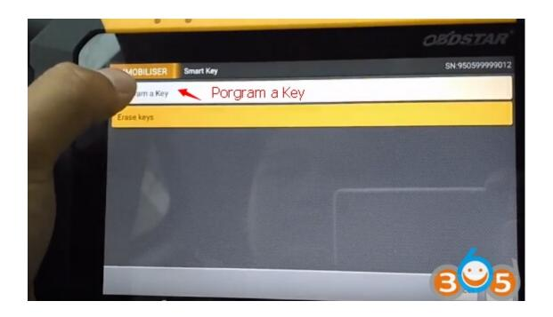
Switch ignition off, press emergency flasher switch OBDSTAR X300 DP will require to enter security code, enter code just read and confirm
