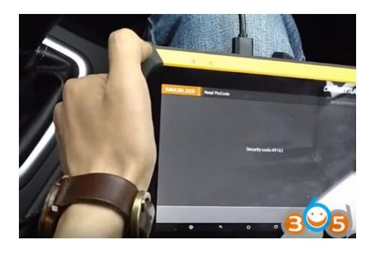
Select mechanical key or smart key to program, here select smart key
